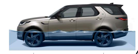
\*Loadspace width will be 1,273mm when 4-zone climate control is fitted. \*\*Dry: Volume as measured with VDA-compliant solid blocks (200mm x 50mm x 100mm). <sup>†</sup>Wet: Volume as measured by simulating the loadspace filled with liquid. <sup>††</sup>Wading depth (25 deg entry and exit) 750mm, deep fording depth (9 deg entry and exit) 900mm. <sup>‡</sup>In off-road height and tow eye cover removed.
